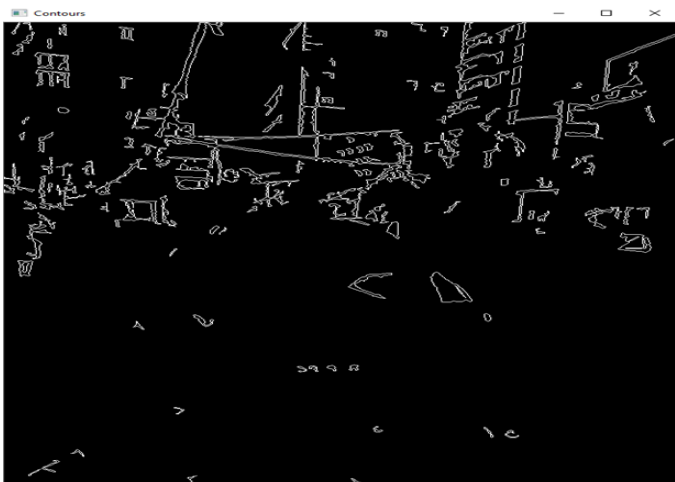
Fig. 20. Contouring to reduce the noise of captured image (Day)
