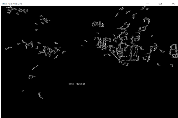
Fig. 27. Contouring to reduce the noise of captured image (Night)
