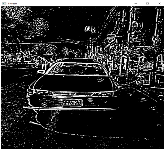
Fig. 25. Thresholding image of the captured image (Night)
