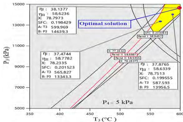
Fig. 11. Overlay plot of most desirable solution
