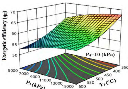
Fig. 6. Effect of  $T_3$  and  $P_3$  on exergetic efficiency ( $\eta_{II}$ )
