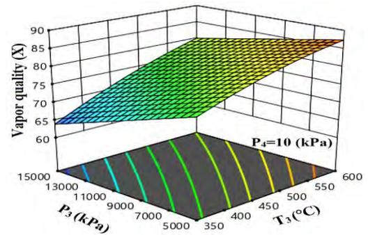
Fig. 8. Effect of  $T_3$  and  $P_3$  on vapor quality ( $x$ )
