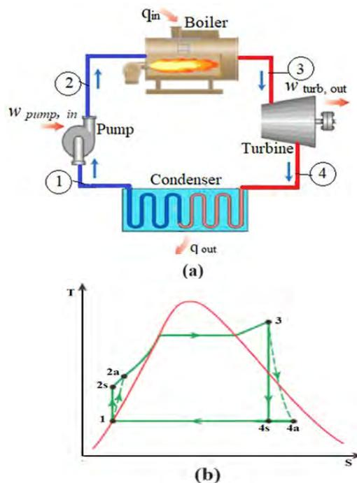
Fig.1.(a) Schematic cycle and (b) T-S diagram of a Rankine cycle
