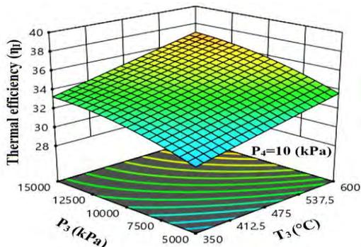
Fig. 4. Effect of  $T_3$  and  $P_4$  on thermal efficiency ( $\eta_I$ )
