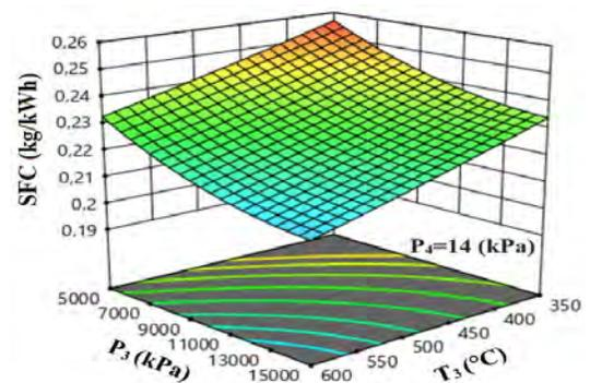
Fig. 9. Effect of  $T_3$  and  $P_3$  on specific fuel consumption (SFC)
