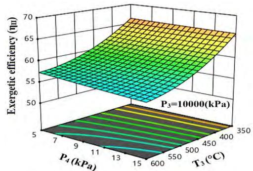
Fig. 7. Effect of  $T_3$  and  $P_4$  on exergetic efficiency ( $\eta_{II}$ )
