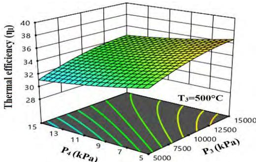
Fig. 5. Effect of  $P_3$  and  $P_4$  on thermal efficiency ( $\eta_I$ )
