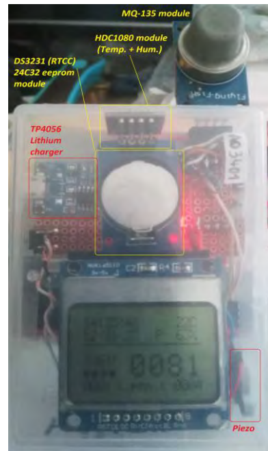
Fig.10: overview of the prototype assembly.
