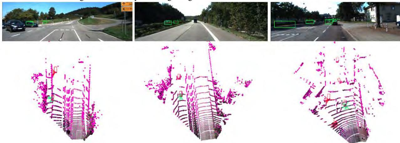
Figure 2: Pedestrian, Cyclist and Car are detected with their assigned bounding box which is green for Car, red for Pedestrian and blue for Cyclist. Object detection done on both images and point clouds.
