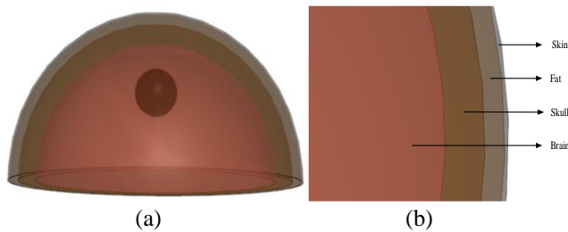
Fig. 3. Human head phantom model, (a) head model with deep seated tumor, (b) four different layers in the head model.
