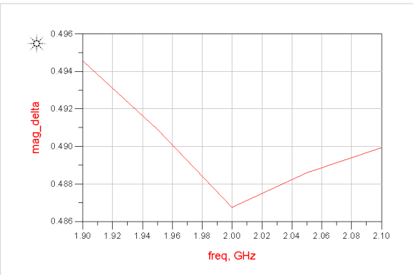
Fig. 15: Delta factor simulation confirms stability.
