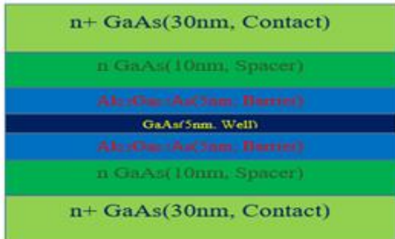
Figure 1: Different layers of the GaAs/Al 0.3 Ga 0.7 As based double barrier resonant tunneling diode [5].
