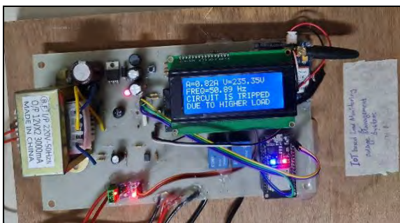
Fig. 13: Circuit Fault Condition while connected with a 200W Bulb
