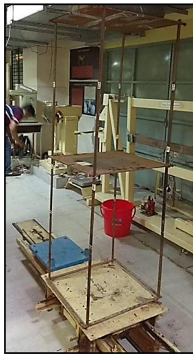
Fig. 2. Prototype of two storied Structural model
