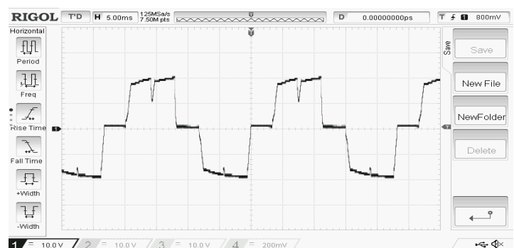
Fig. 11: Line to neutral voltage for inductive load for 180° conduction mode.
