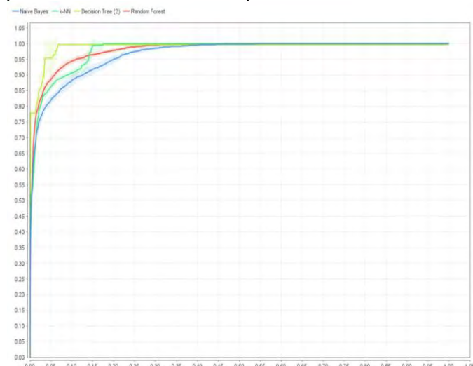
Fig. 14. Compare ROCs curve of Decision tree, Naive bayes, k-NN and Random Forest classifier.
