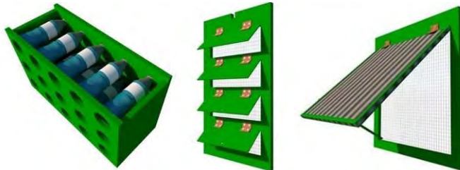
Fig 10: Proposed ventilation and opening modules
