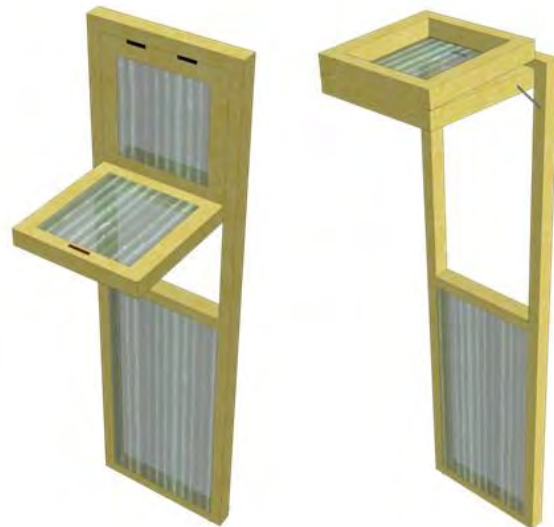
Fig 13: Composite opening module made of semi-transparent polycarbonate sheet placed in wooden frame, having a foldable opening part to fit into spaces with minimum setback
