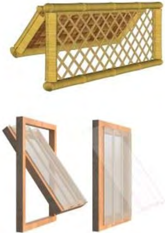
Fig 15: Ventilators made of bamboo with pivot type shutter and Pivot type openings made of polycarbonate sheet in wooden frame
