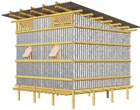
Fig 14: Proposed dwelling unit after retrofitting with pivot type openings and ventilators with pivot type shutter
