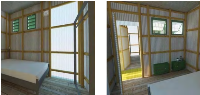
Fig 09: 3D visualization from inside, showing the room is illuminated by using semi-transparent polycarbonate sheet and well ventilated by using awning type windows along with louvered openings and exhaust fan as active ventilator.
