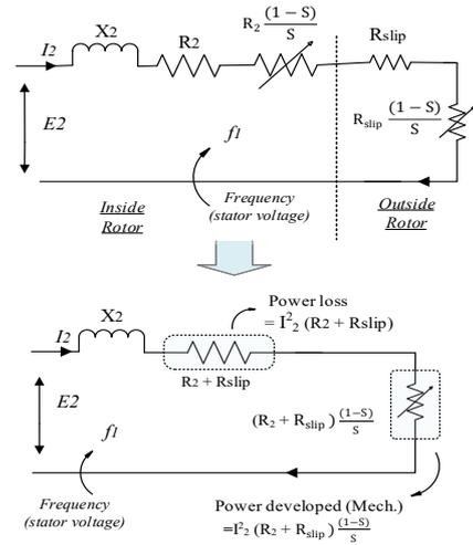
Fig. 3. Modified rotor equivalent circuit of SRIM with slip resistance and various power components
