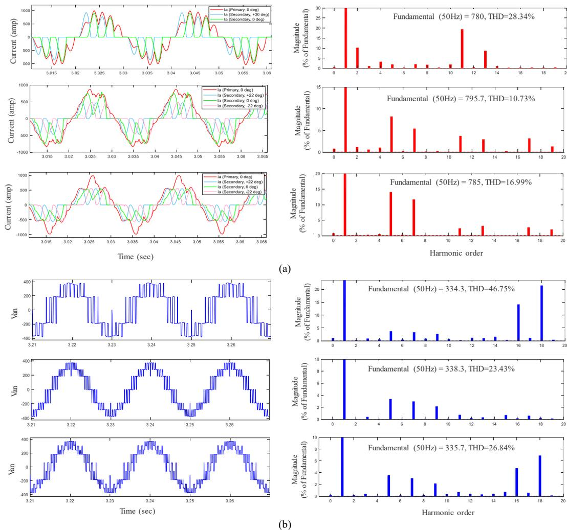
Figure 9. (a) Simulation results for the input current with harmonic spectrum. (b) Simulation results for the inverter output voltage with harmonic spectrum; (top) 12-pulse rectifier with two-level inverter, (middle) 18-pulse rectifier with three-level inverter, (bottom) 18-pulse rectifier with four-level inverter
