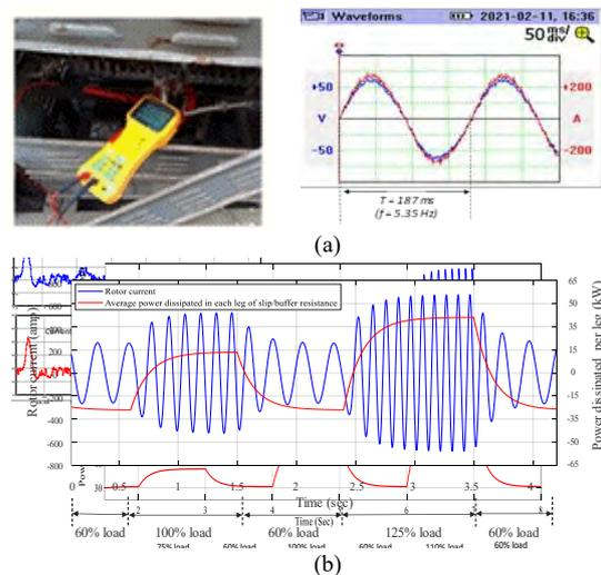
Fig. 4. (a) Voltage and current for one leg of slip resistance. (b) Simulation results for rotor current and average power loss (per phase)
