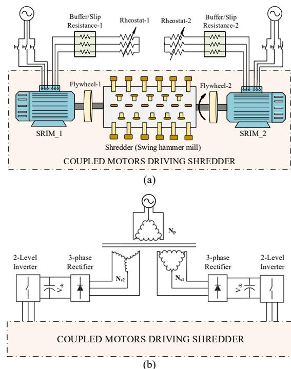
Fig. 1. Existing two types of electric drives for sugarcane preparation (a) SRIM drive. (b) 2-level inverter based VFD.
