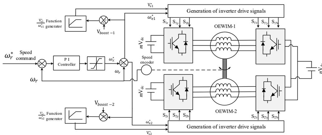
Fig. 8. Closed loop volt/hertz control scheme for the proposed OEWIM drive
