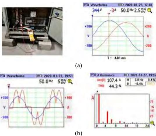
Fig. 6. (a) V(phase) and I(line) for SRIM drive. (b) V(line) and I(line) for VFD and harmonic spectrum of current
