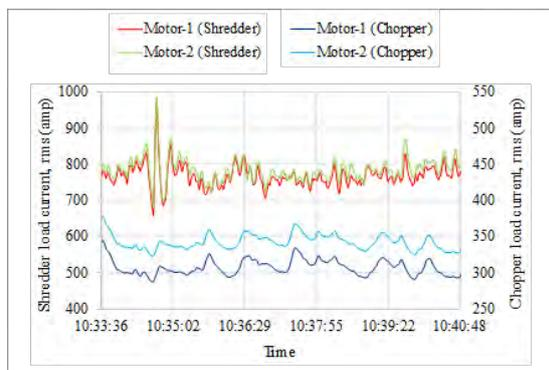
Fig. 5. Load current(rms) by coupled SRIM drive and VFD of a sugar factory obtained from DCS.
