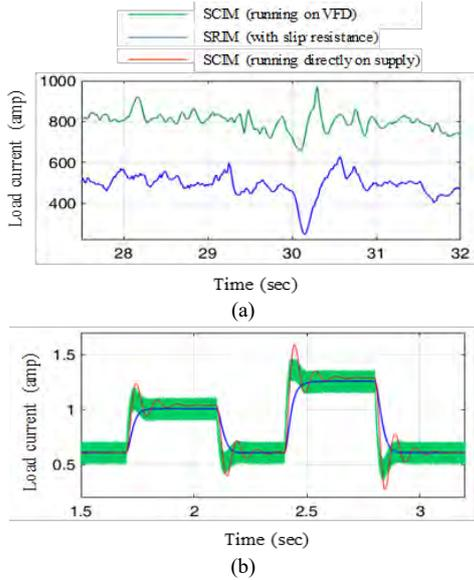
Fig. 2. (a) Load current (rms) for shredder and chopper obtained from the DCS. (b) Simulation results for load current during impact loads.
