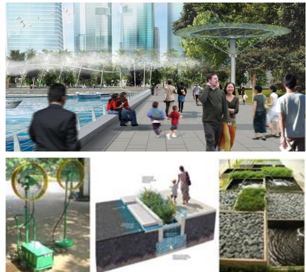
Fig. 4. Streetscape elements- water fountain, mist fan and rain garden installed to achieve passive cooling in tropical urban areas
