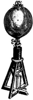
Fig. 4. Designed Piston vacuum pump from 1658 to 1659 by Robert Boyle and Robert Hooke.
