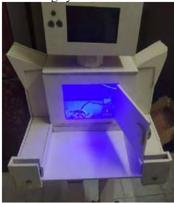
Fig. 15. Sterilizing the equipment via UV-C light.
