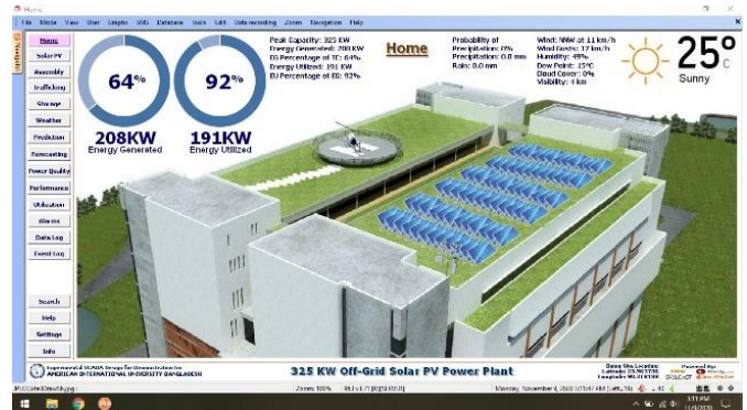
Fig. 5. Supervisory Control and Data Acquisition (SCADA) Graphical User Interface (GUI) implementation.
