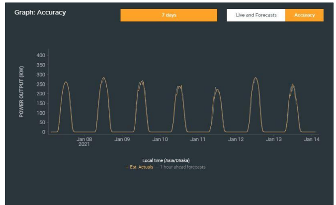
Fig. 16. Solcast simulation results of supply prediction showing accuracy report for 7 days.
