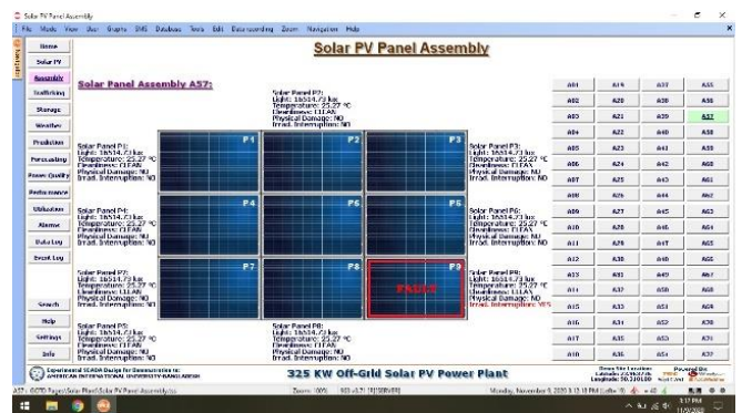
Fig. 7. Individual assembly monitoring page of SCADA GUI.
