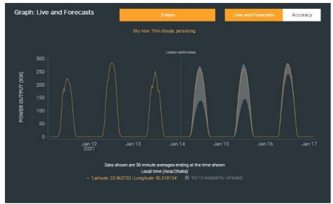
Fig. 15. Solcast simulation results of supply prediction showing live and forecasts for 3 days.
