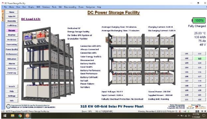
Fig. 9. DC power storage facility of existing online UPS monitoring page of SCADA GUI.
