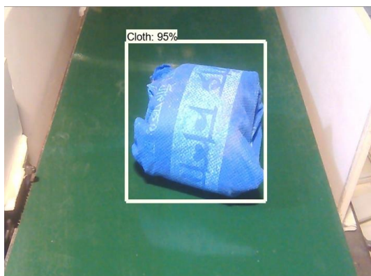
Fig. 16. The detection of cloth using machine learning technique
