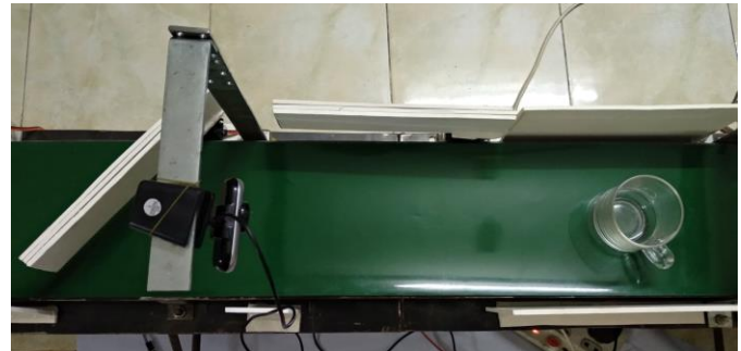
Fig. 13. Closing of the gate after the detection of glass
