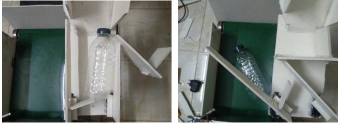
Fig. 10(a) Object at the end of the funnel Fig. 10(b) Dropping of object on the conveyor from the funnel
