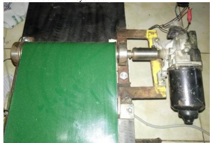
Fig. 9. Implementation of the wiper motor on the system
