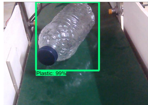
Fig. 14. The detection of plastic using machine learning technique.
