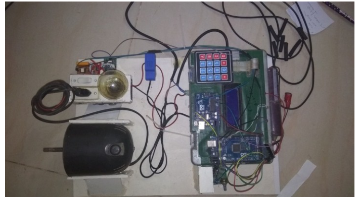
Fig. 5: Primary experimental set up for SBMS Energy Management System
