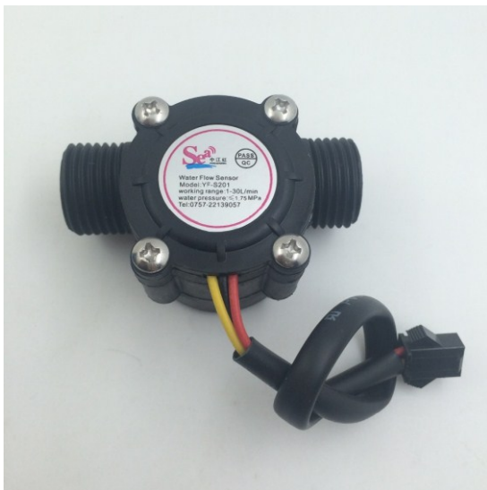
Fig. 6: G1/2" Water Flow sensor (Model - SEN-00043) for SBMS Water Management System [18]
